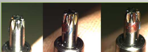
Highlighted soiling on the half of the same gear, due to the non-internal rotation of the HP (halves separated by blue spot)
