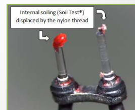
Control test : highlighted interest of pushing a nylon thread through the air/water pipes
